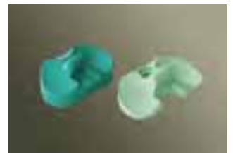
TECAFORM AH MT Sizing trials for knee implants.
